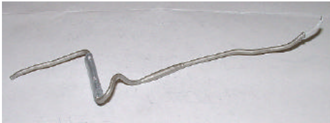
Trimmed and assembled exhaust with header pipe.
